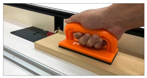
Place the push block on a flat piece of stock and a safe distance away from the Cutter. Apply pressure downward and inward toward the fence. Slowly and steadily feed the stock through the cutter until the cut is completed.
