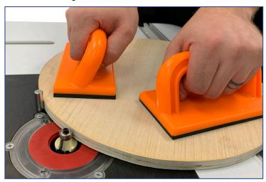
When using your router table to mill round stock, it can be a little dicey as for as safety goes. With two push blocks, you can control your stock while keeping your fingers safely away from the cutter.
