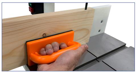
When re-sawing stock on the band saw, a push block can be the perfect way to feed your stock through. The push block grips your stock, all the while keeping your fingers safely away from the running band saw blade.
